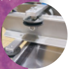
Horizontal wheel and track system locks the machine onto the table, which absorbs any residual vibration. The horizontal wheels are fully adjustable (an APQS exclusive) to eliminate play.
