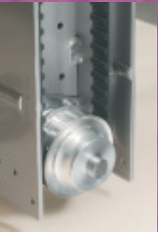
Synchronous belt drive technology provides precise machine timing.
